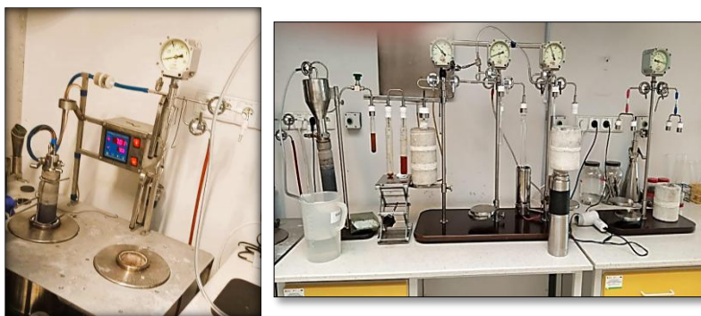
Fig. 2 Benzene line at Gliwice ^{14}\text{C} and Mass Spectrometry Laboratory.
